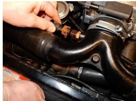
Remove the 4 screws holding the Throttle body onto the intake plenum.
