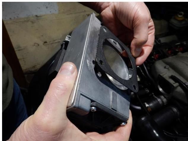
It is normal for the car to generate an error when first started with a new ETM, and so this should be cleared and the errors will not re-appear. I think the ECU learns the ETM settings in some way, so when it first starts with a different ETM it assumes its an error.
