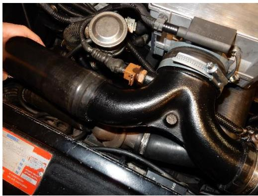
Remove the two large rubber hoses from the intercoolers by removing the securing clips and pulling them off.
