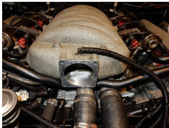
Fitting your new Throttle body is a reverse of this procedure. Do not overtighten the mounting screws as the plenum body is aluminium and so you can damage the plenum.
