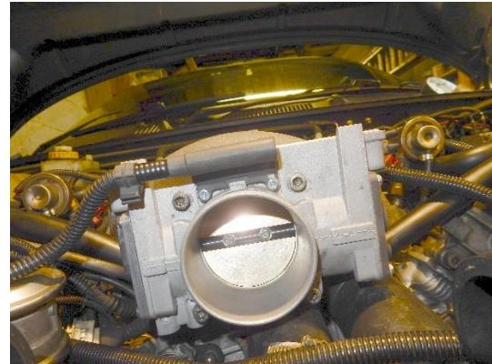
You should now be able to remove the Throttle body. Depending on how long it has been there and whether gasket sealant has been used it may take a little pressure to remove it.
